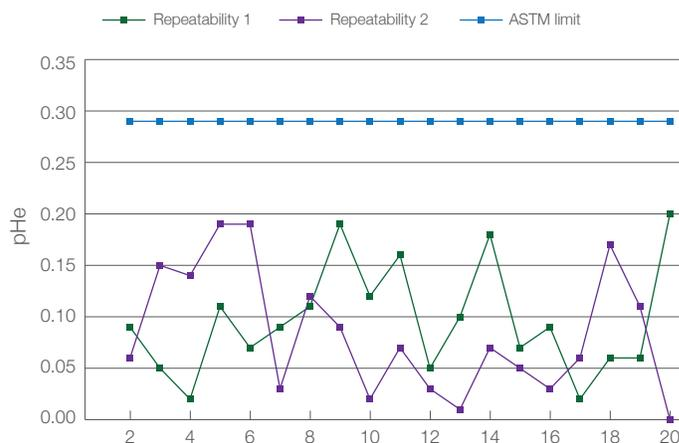
As shown on the chart above, the repeatability of successive measurements of twenty ethanol fuel samples by the Orion 8172BNWP electrode is in accordance with the ASTM D 6423-08 Standard; the biggest deviation between successive results is 0.29 pHe or less.
