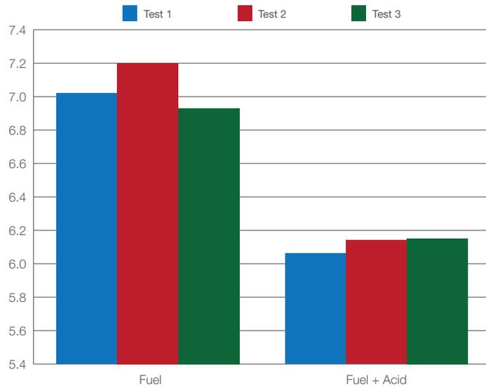
When cycling between fuel and acidified fuel, the Orion ROSS Sure-Flow electrode showed good repeatability and was sensitive to the acid additive.
